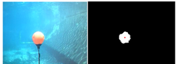
Fig. 18. Original Image and Processed Image for Buoy Detection
