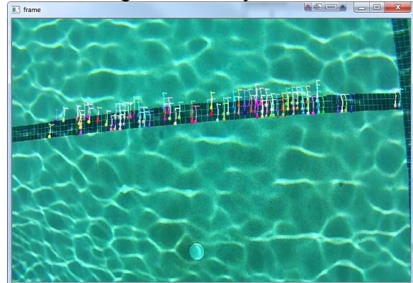
Figure 18 - Optical flow displaying motion vectors
