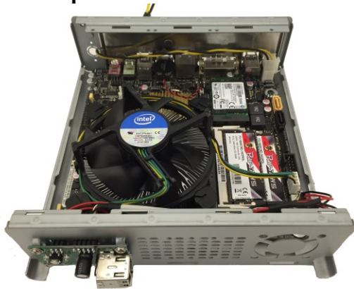
Figure 8 – Computer case with Cover Removed
