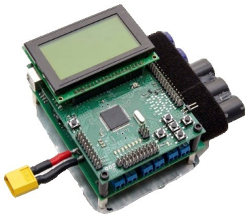
Figure 11 - Main Interface Board
