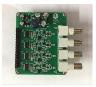
Fig. 1.1 hydrophone signal processing module
