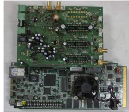
**Figure 11:** *Custom Designed Acoustic board integrated with DSP Evaluation Board*
