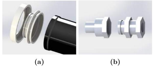
**Figure 3:** (a) Design of End Cap for Battery Pod; (b) Connectors
