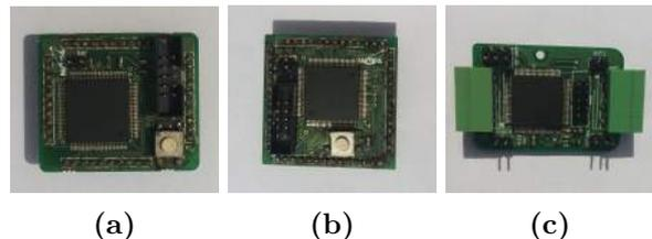
**Figure 9:** *Power, Motion Controller and Pressure Sensor Boards*
