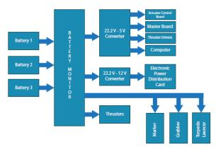
Figure 8. Electrical system block diagram[2]
