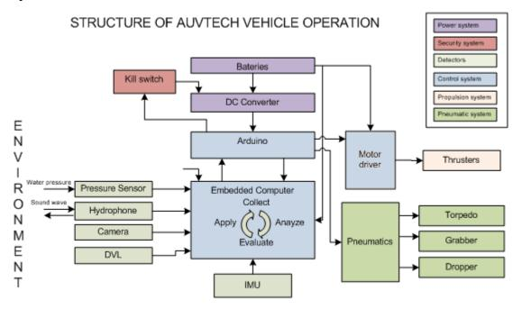
Figure 2. AUVTECH Sub-systems and their interactions.
