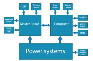
Figure 7. Electrical system block diagram[1]
