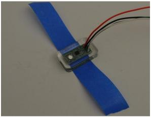
Figure 10. Depth sensor
