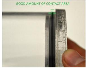
Figure 4. Plexi endcap with o-ring
