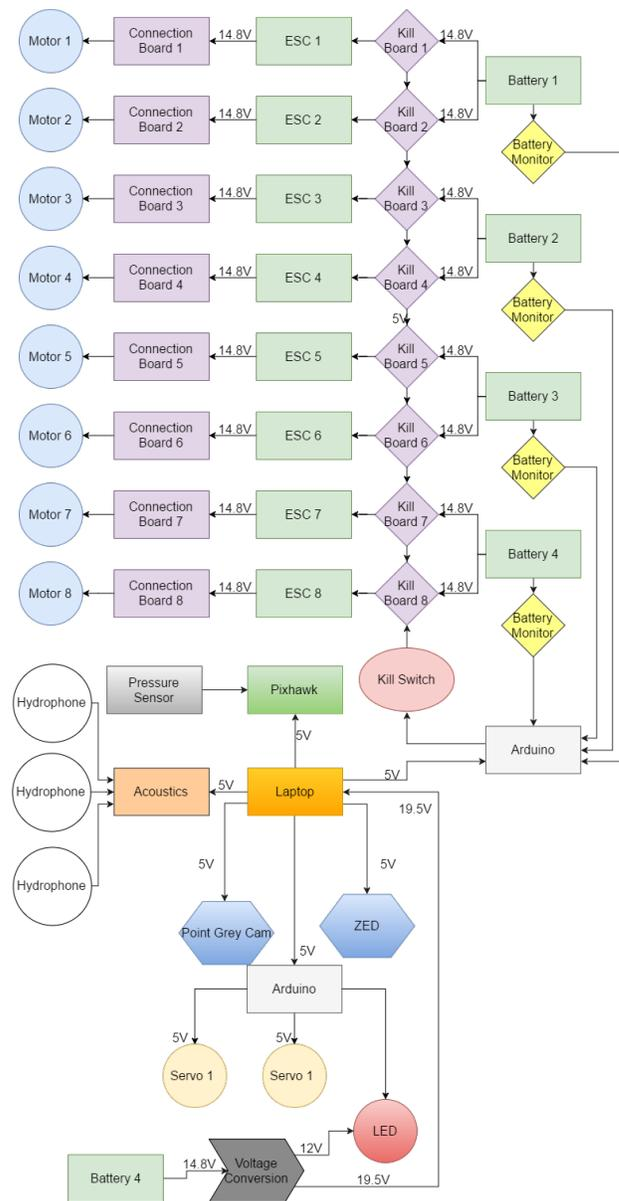
Fig. 5: Electrical Wiring Diagram
