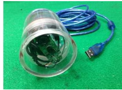
Fig. 27. Under water monitoring Camera
