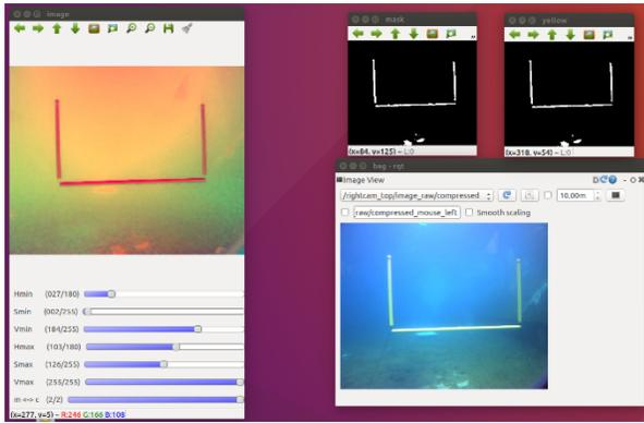
Fig. 22. Vision system interface for gate detection.
