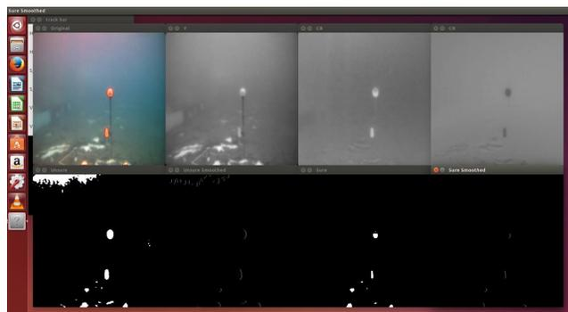
Fig. 21. Buoy in YCbCr color space.
