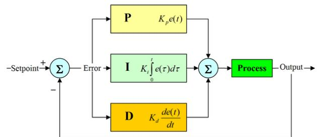
Fig. 17. Block diagram of PID control algorithm
