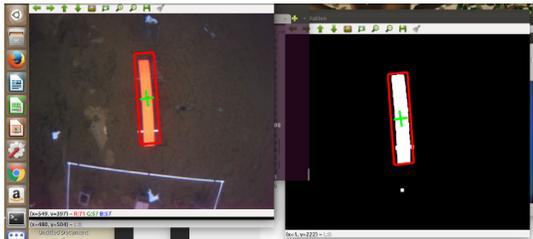
Fig. 24. Shape detection for path determination task.
