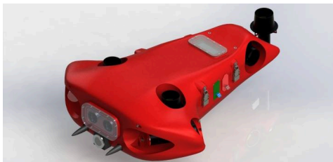
Figure 2: A concept image of the design of Naiad from Solid Works.
