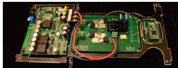
Fig. 10. The power supply, power distribution board, and Teensy shield all fit on the top rack inside the main hull.
