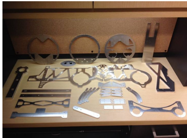
Fig. 6. Bixby's frame is made entirely of anodized aluminum.
