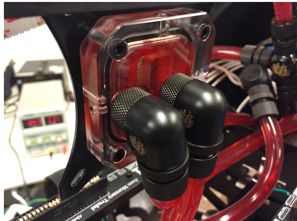
Fig. 4. Bixby's CPU is cooled using a custom water cooling system.
