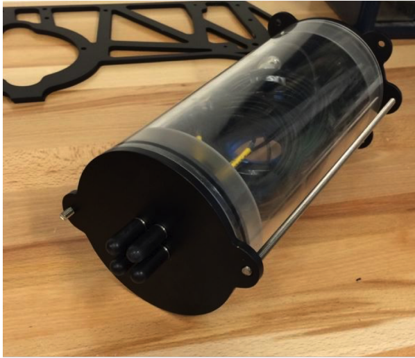
Fig. 5. Array of four hydrophones.
