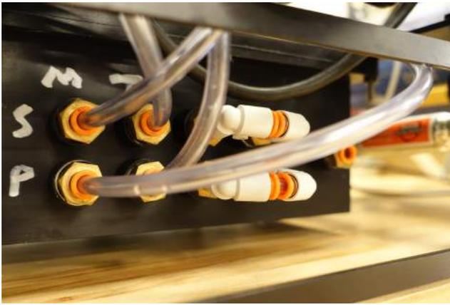
Fig. 6: Pneumatic valve housing
