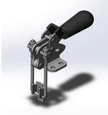
Figure 8: A part model of the toggle clamps which will be used to secure the end cap.
