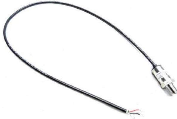
The pressure sensor in Sanka is a p51 media sensor pressure sensor and allows the sub to know what depth it is at. It interfaces with the arduino microcontroller which takes the raw data and turns it into a useful depth reading. It is molded into the end cap so that it is in direct contact with the surrounding water. Without the pressure sensor, the sub would not be able to control or maintain a depth.
