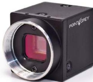
The Sanka uses two external cameras that connect to the motherboard using the USB 3.0 ports. The top camera is a Flea3 that is housed in a waterproof case. The bottom camera is a Microsoft HD life cam studio camera. These cameras allow the sub to control itself based on its surroundings using a visual interface. The cameras can be used to find colors and accurately shoot torpedoes. These cameras allow Sanka to find and complete missions, and are essential to the sub.
