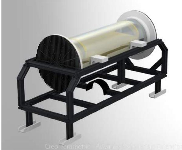
Figure 9: An assembly drawing showing the raised frame design and the PVC mounts.
