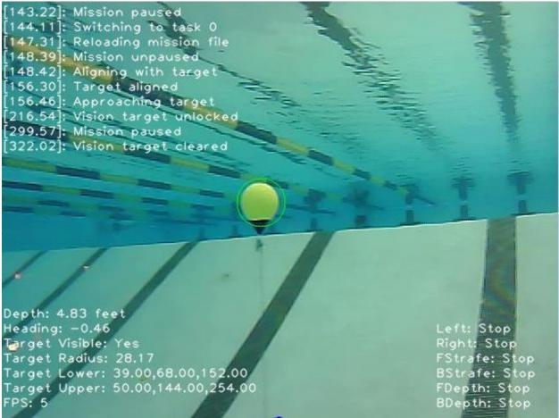
Figure 12 – Program running with view from front camera while tracking a buoy
