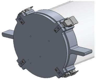
**Figure 3** – Solidworks model of the rear endcap with latch mechanisms
