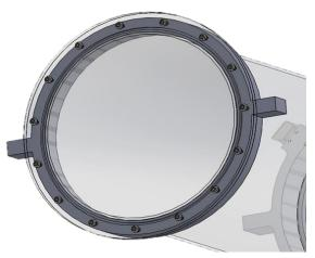
Figure 4 – Solidworks model of the clear front end cap
