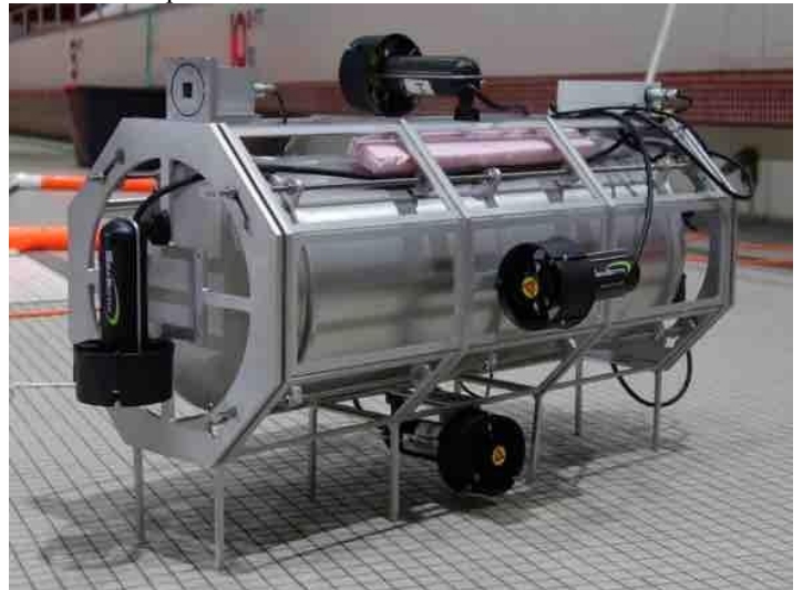
Fig. 3. Seawolf VI, fully assembled frame and hull with thrusters
