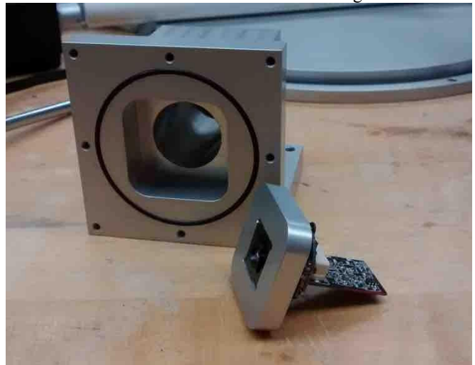
Fig. 8. Camera and Camera Enclosure
