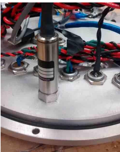
Fig. 7. Pressure transducer mounted to the end-cap
