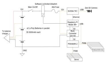
Fig. 1. Electrical Diagram
