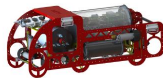
Fig. 1: A Solid Works Rendering of Paxer
