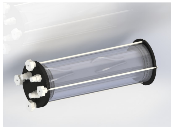
Fig. 5: A SolidWorks Rendering of Nemo Carrot's Battery Pod
