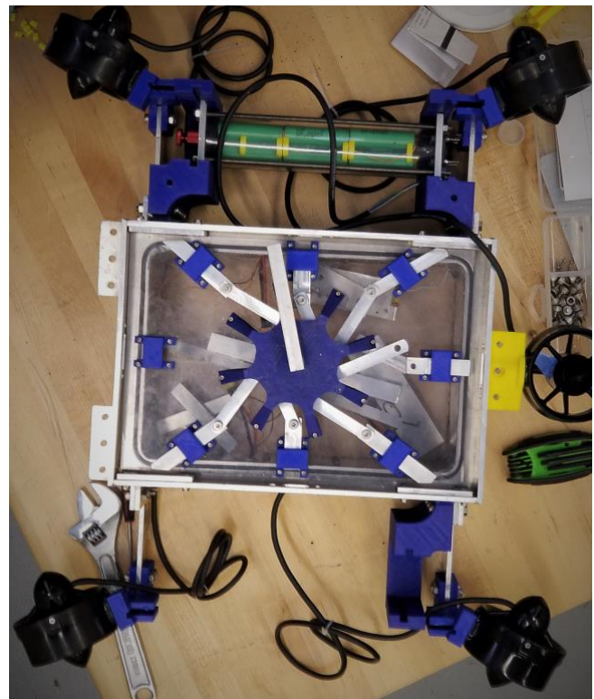
Fig 11. Sub with top-down view of bank vault style lid
