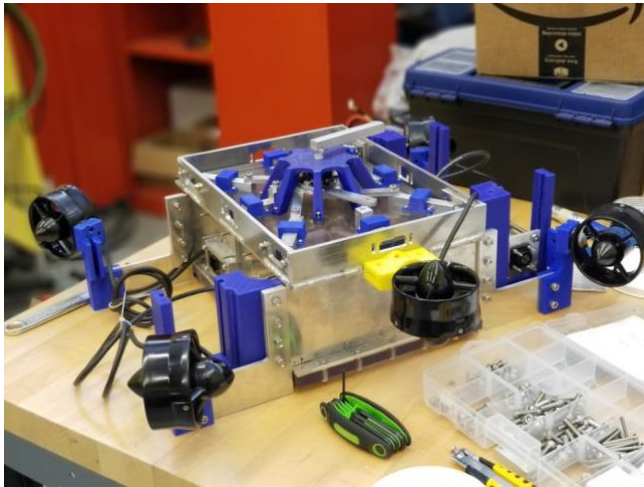
Fig 16. Final Hull with all thrusters
