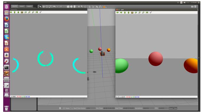
Fig. 7. Example of simulating the stereo camera system in Gazebo. Pictured is a disparity image (left), the simulated scene (center), and the raw image from the simulated left camera (right).
