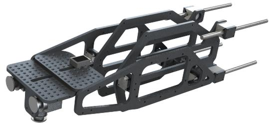
Fig. 4. CAD rendering of *Riptide's* previous electrical mounting system.
