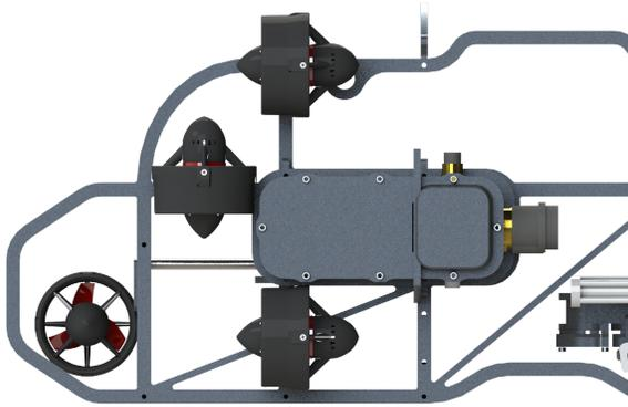
Fig. 3. Close up of the updated thrust placement on *Riptide's* chassis.
