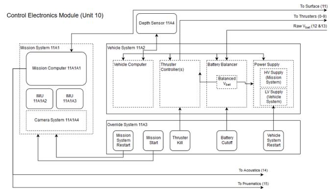
Fig. 2. Block Diagram of *Riptide*'s custom electrical system.
