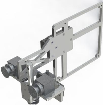
Fig. 6. Close-up of a CAD rendering of motherboard mounting system, with cameras in place.
