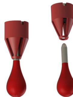
Fig. 5. CAD rendering of marker dropper system.
