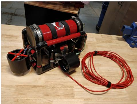
Fig. 7. STEMbot, UWRT's remotely operated vehicle.
