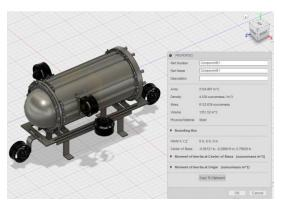
Fig. 16 Autodesk Fusion Rendering of Center of Buoyancy Calculations
