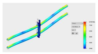
Fig. 14 Von Misses Stress Analysis of Camera Rods with Rod Clamp
