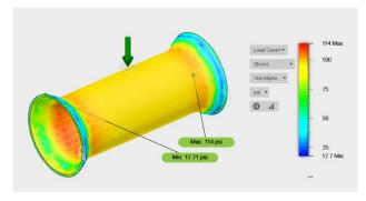
Fig. 3 Stress Analysis for the Hull
