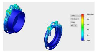
Fig. 8 Stress Analysis of the Front and Back Endcaps
