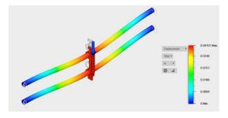
Fig. 15 Displacement Analysis of Camera Rods with Rod Clamp
