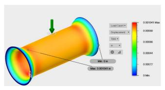
Figure 4. Displacement Analysis for Hull
