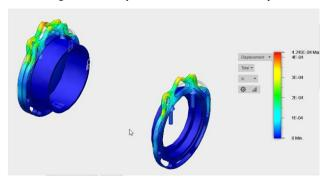
Fig. 9. Displacement Analysis of the Front and Back Endcaps
