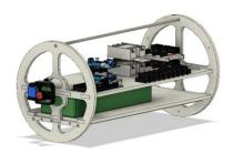
Fig. 13 rendering of a Delrin bases Electronics Rack
