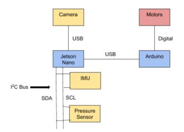
problems with PWM over the GPIO pins of the Raspberry Pi, so we chose to use an Arduino this year for our PWM needs, a system with which we are more familiar. A diagram of our data flow is shown below.
