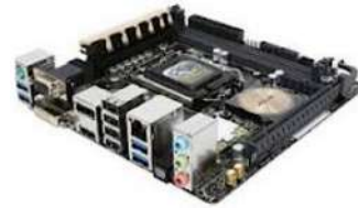
Figure 13: Sub's main computer – ASUS mini-ITX
