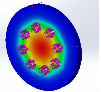
Deformation fringe plot of the aluminum 6061-T6 Rear Bulkhead, water side.
