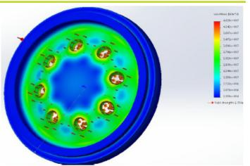
Stress fringe plot of the aluminum 6061-T6 Rear Bulkhead, Housing side
