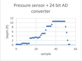
Fig 5. First useful data after debugging electronics.
