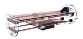
*Fig 4. A Rendering of the AUV's Central Compartment.* A major refit was performed on the way components
