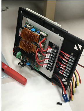
Fig 11. Power Board Mounted on 3D Printed Tray
