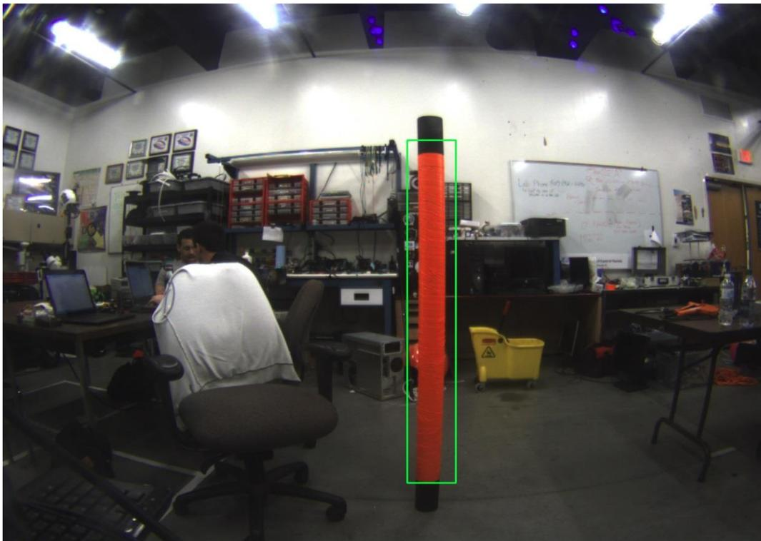
Figure 2: Object detection detecting a pole in the scene using color thresholding visual saliency.
