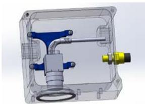
Fig 8. External camera pressure vessel with PoE camera.
