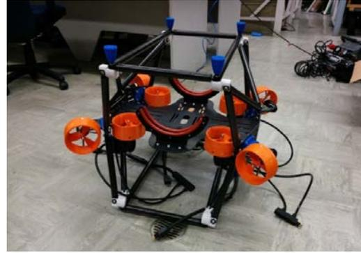
**Fig 3.** Hybrid carbon fiber and sheet metal framework with thrusters attached. Note the vectored thruster layout.
