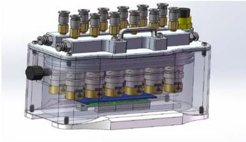
Fig 11. Pneumatic solenoid housing and control board.
