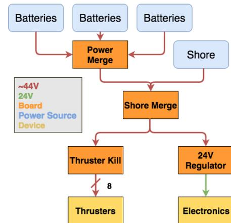
Fig 6. Power flow diagram.
