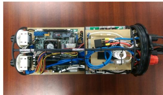
**Fig 4.** Internal electronics carriage for the main vessel. Above the tray there is easy access to PCBs and wiring, while batteries are stored below the tray.
