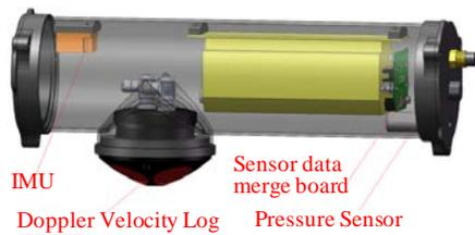
Fig 7. Model of the navigation vessel (transparent for viewing).
