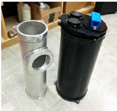
**Fig 2.** Navigation vessel before anodization (left) and main vessel with front endcap (right).
