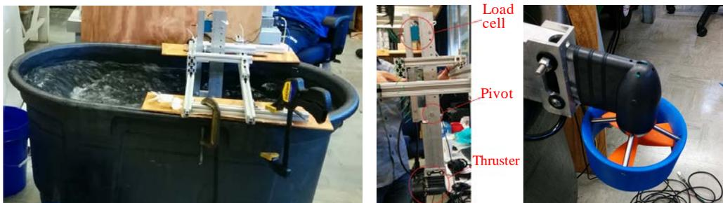
Fig 10. Thrust test (left), apparatus (middle), and current propeller/nozzle design (right).
