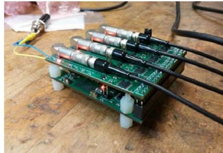
Fig 9. Passive sonar amplification and processing hardware.
