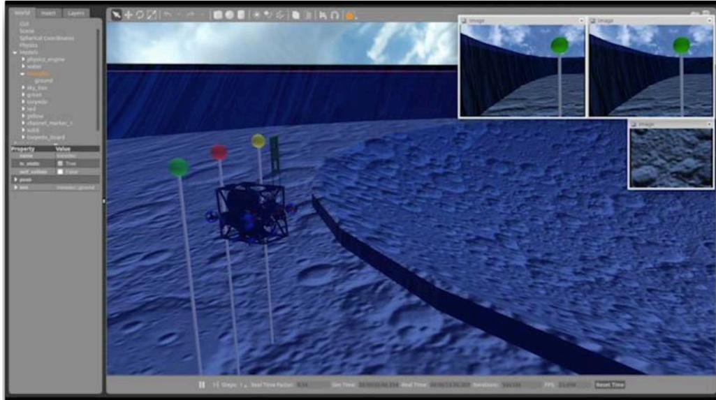
**Fig 16.** Sample simulation showing output from onboard cameras.
