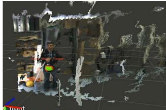
Fig 14. Stereo point cloud generation.
