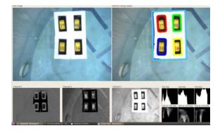
Figure 7: Bins positions are identified by the vision system
