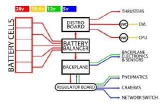
Figure 5: Power Distribution Layout
