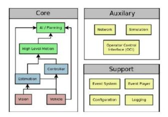
Figure 8: Tortuga V Software System Diagram
