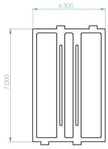
Figure 2: Basic external frame panel design
