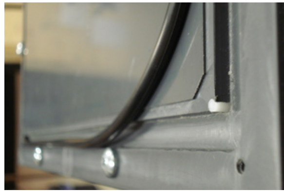
Figure 3: O-ring displaced to show the grooves and nylon dowel.
