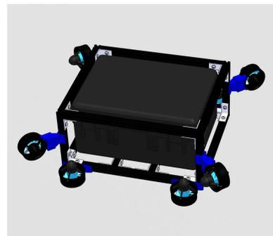
Figure 2: BLOCK 1, the first testing rig for the 2018-2019 year consisting of a large waterproof case with a frame of aluminum extrusions
