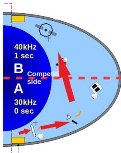
Fig. 1: The course plan for Seahorse (in red). Seahorse's main goals are passing through the gate, hit the buoys, and surface.
