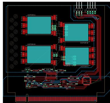
*Figure 4: An example schematic of a custom PCB from the first stage of development, designed to be plugged into the edge connectors of the main bus.*
