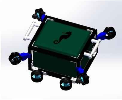
*Figure 3: BLOCK III (Seahorse), the latest vehicle for 2019. The body consists of a small waterproof case, aluminum extrusion frame, 3d printed thruster mounts and steel handles.*
