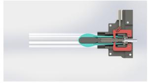
Figure 3 Torpedo launching mechanism
