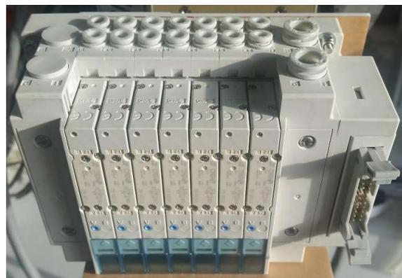
Fig. 5. SMC SY3100 U1 solenoid valves
