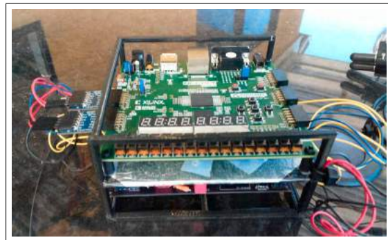
Figure 6: FPGA with hydrophone circuits
