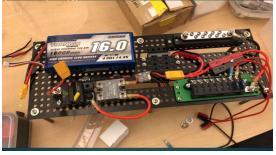
The electronics system was thoroughly benchtop tested before pool testing. We created FlatSub (left), a 1-for-1 replica of the electronics system that was used to prototype and test each component under load and failure conditions before integration into the robot. We estimated the peak continuous load to be around 40A and designed the electronics to handle 80A continuous current. We tested the custom circuitry and safety switches under a full thruster
