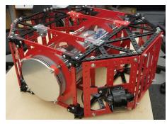
The physical structure of Seawolf VIII consists of multiple 0.25 in thick 6061 aluminum frame sections held together by 3D printed joints and stainless fasteners. The aluminum frame is an improvement on Seawolf 7's design as the acrylic frame of SW7 was fragile and led to many mechanical issues, whereas SW8's design provides structural integrity and prevents external forces from acting on the electronics hull where possible.
