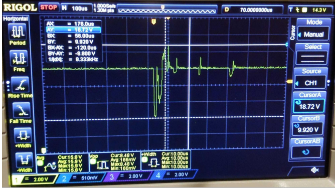
Fig. 8. Noise from inrush current
