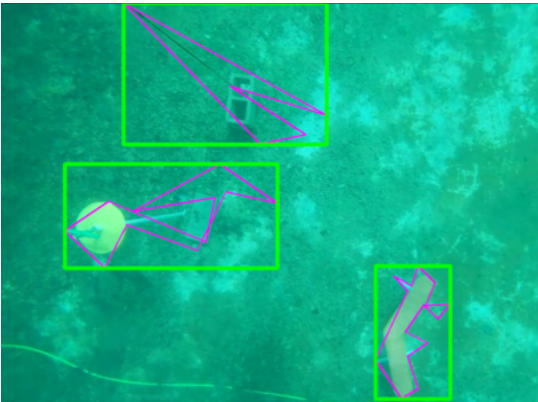
Fig. 6. Largest objects are detected after filtering. HSV filtering will next be applied to remove objects that do not match the color profile of the path markers.
