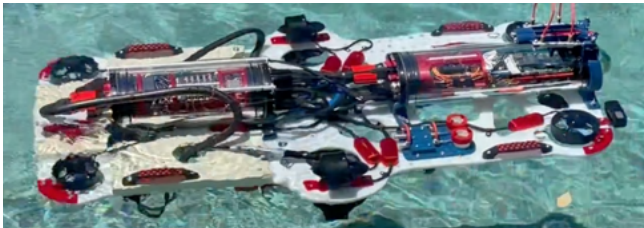
Fig. 9. Buoyancy test of Dragon with foam and its final frame constructed out of HDPE.
