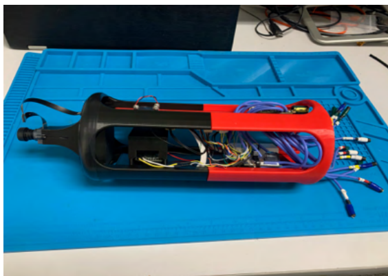
Figure 4: Electronics in custom 3D printed enclosure
