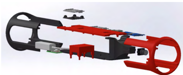
Figure 3: Exploded view of our custom 3D printed enclosure mounting system
