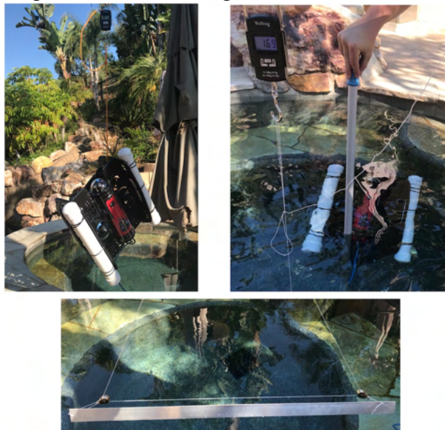
Figure 11: Center of gravity and center of buoyancy testing
