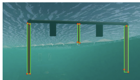
Fig. 5. OpenCV code identifying the gate on live video feed from the Unity simulation.
