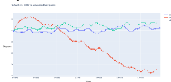
Fig. 4. Graphed data of the PixHawk IMU (red) and AHRS heading values (blue and green). PixHawk values seem to drift significantly. Values from the AHRS devices had a better accuracy of \sim 0.8^\circ
