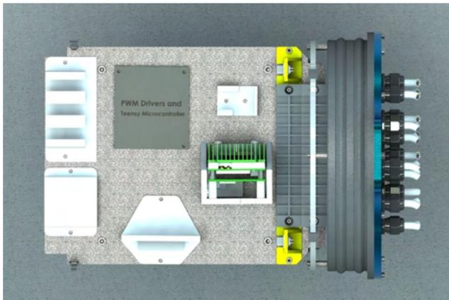
Fig. 3: Overhead view of the mounting plate and component mounts.
