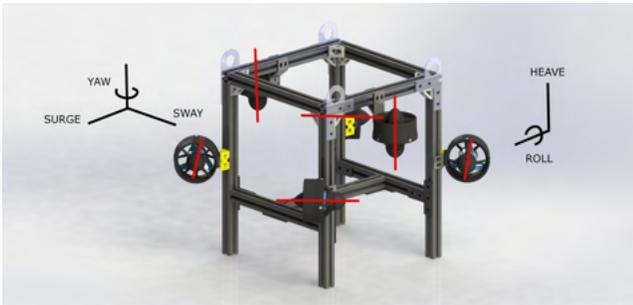
Fig. 4: AUV thruster layout illustrating degrees of freedom
