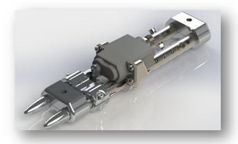
The dropper module is also homemade. A magnet located on the inside of the enclosure is pulling on another magnet on the outside of the enclosure until the inside magnet is rotated 180° apart by means of a servo. This action pushes out
