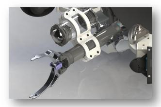
The torpedo launcher is a custom design that uses a servo motor as a trigger. The launcher also has two torpedoes centered under a camera to make it easier to aim. Both those characteristics make the launcher simple to integrate with the whole system and its function's reliability is improved by its chosen placement.
