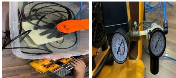
Figure 23 Enclosure testing; Compressor pressure regulator
