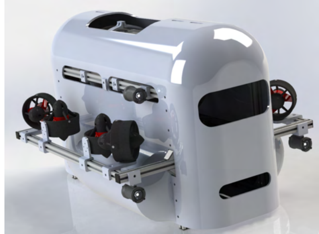
Fig. 1. Render of AUV Beluga created in SolidWorks.
