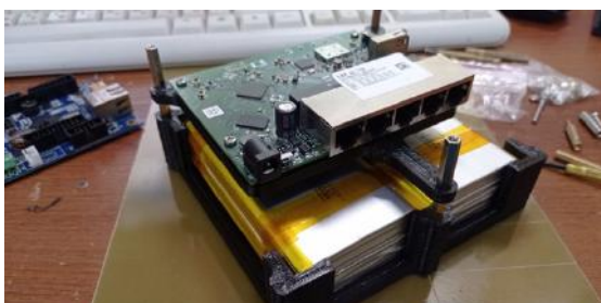
Figure 5 "Battery pack and Ethernet switch"
