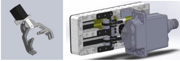
Fig. 4: BBAUV 4.0 Grabber and Torpedo Launcher.
