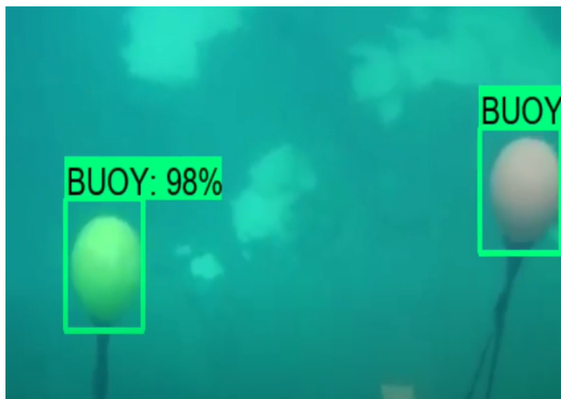
Figure 8: AI Vision System determining buoy confidence and location in relation to ANDY.
