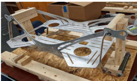
Figure 4: SubjuGator 9 Aluminum Chassis
