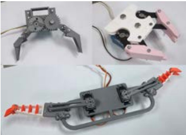
Fig. 6: Basic (a), Parallelogram (b), and Track (c) Claw Prototypes
